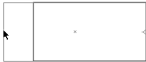
Drag-scaling Uniformly (Side point of origin shown)
